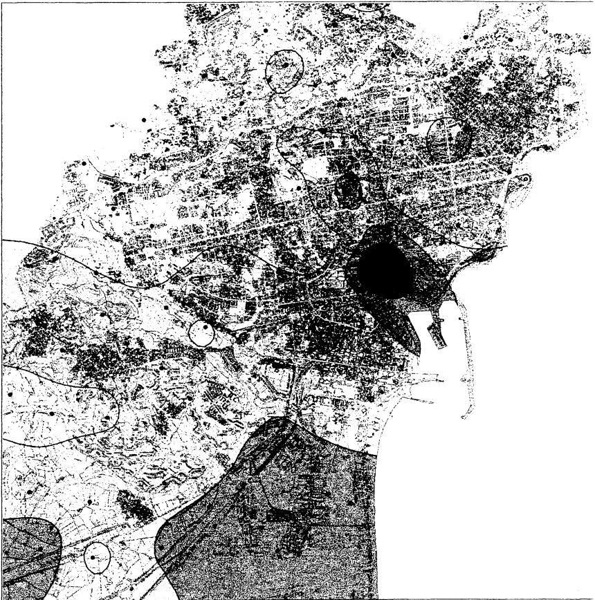
Figure 1: Distribution of the values of the synthetic 5% pseudo-acceleration spectra taken at 5 Hz in the urban area of Catania. Higher values correspond to the darker zones.
